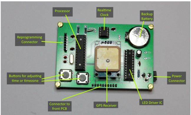
I like to solder the smallest parts first (the parts that stand shortest on the board), moving on to the larger parts later.
