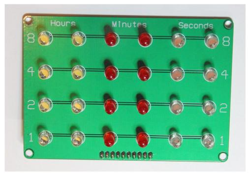
Note that LEDs must be soldered the correct way around. If you look at the silk screen (the white markings on the PCB) you'll see that each LED has the positive pad marked with a "+" symbol. The **longer** of the LEDs two legs should go in here.
